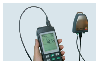
Inspection of transmitters with 4 to 20 mA interface
