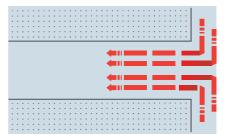
Exhaust air: In the case of exhaust air outlets, the air is drawn in from all directions. To generate an air flow that can be measured accurately, a funnel must therefore be used. Compatible measuring instruments testo 440 100 mm Vane Kit with Bluetooth (order no. 0563 4403)
