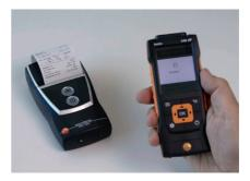
With the IRDA/Bluetooth printer from Testo, you can print out the measurement results of the testo 440 directly on site, wirelessly, in the form of a report to hand over to the customer or to store in your records.
