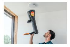
The testovent 417 measurement funnel allows you to measure at standard supply air outlets more accurately and, above all, faster. The funnel therefore enables you to measure with more speed and accuracy.
