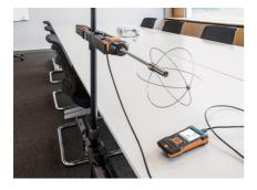
If there are indications that people perceive the air flow to be unacceptable or if noticeable effectiveness of air terminal devices is determined or can be expected, this condition can be assessed objectively by determining the degree of turbulence and the draught risk. The appropriate measuring instrument, with a turbulence probe, measures air velocity and air temperature and automatically calculates the draught risk and degree of turbulence.
