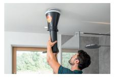
A funnel is essential for measuring the exhaust air. The reason: there is no directed flow profile available for exhaust air as the air is sucked out of the room in a funnel-like pattern. This means there is no definable area in the room from which the volume flow can be determined. This challenge is easily solved with the aid of the testovent 417 funnel. This is because the funnel creates defined flow conditions at some distance from the plate outlet in a fixed cross-section.
