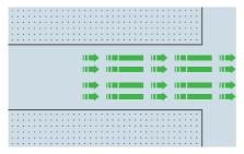
Supply air: In the case of supply air outlets, there is a directed air flow, which you can accurately record using the testo 440 and compatible vane anemometer.
