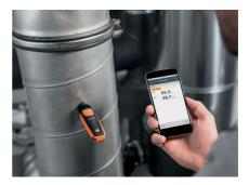
When determining the air temperature in ventilation ducts, the measuring probe also has an effect on the result. Heat conduction and turbulence can significantly falsify the measurement result. For this reason, special attention must be paid to the immersion depth and position of the probe in the air flow:
