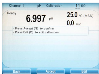
Example 3: When the pH buffer reading is stable, onscreen text prompts and function keys update with the appropriate instructions and options.
