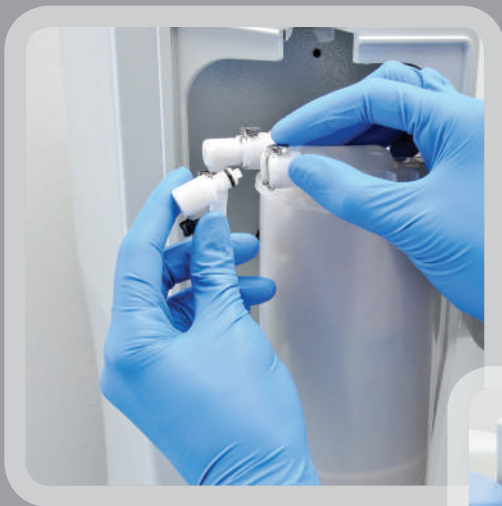
Quick-connect cartridge replacement
