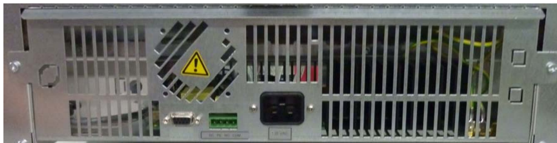
Figure 5-10 AC Power Supply Socket
