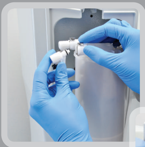
Quick-connect cartridge replacement
