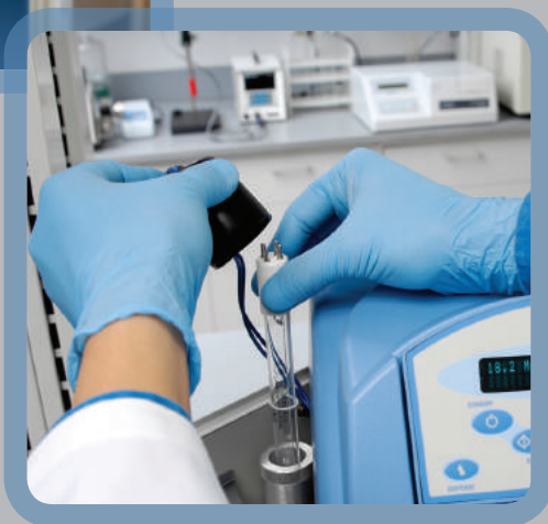
Changing the UV lamp protects the system against microorganisms and oxidizes organic compounds in the feed water, allowing for TOC levels of less than 5ppb
