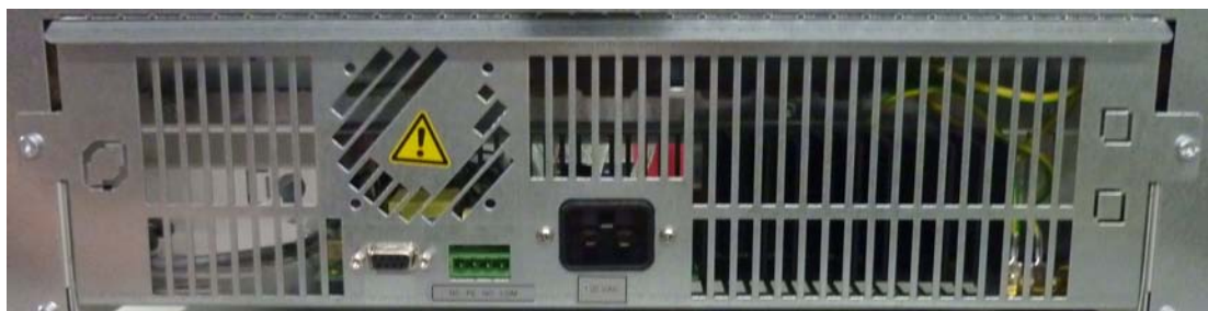
Figure 4-16 Signal Interfaces and Power Socket
