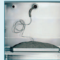
Interior chamber with flexible Pt 100 temperature sensor in granulate sample
