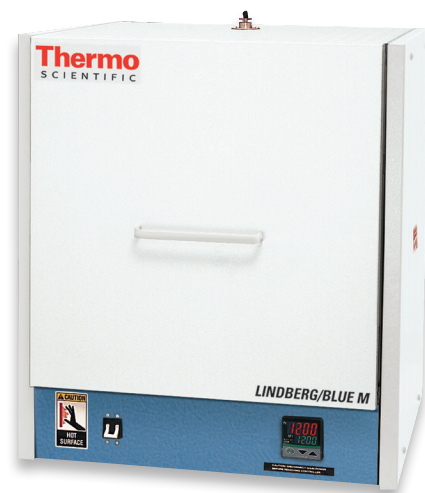
Model BF51842C-1 with horizontal side swing door
