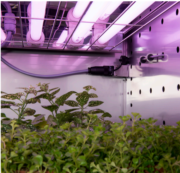
Interior of Forma Vertical Light Chamber with plant growth light modules installed.
