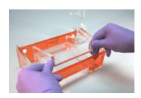
2. Pour warm (<60°) agarose onto tray and set combs in the desired comb slot(s).
