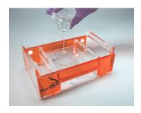
3. Once solidified, turn the tray 90 degrees to the running position, remove combs, add buffer, load samples and run the gel.
