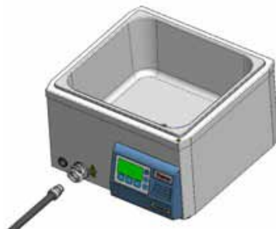
Figure 3-3 – GP Bath Drain Hose
