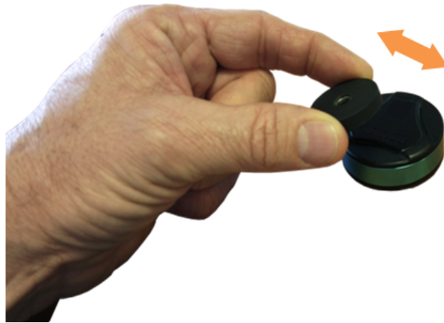
Figure 6. Check status by holding magnet over module
