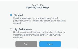
Figure 24. Operating Mode Setup Screen
