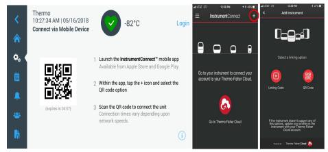
**Figure 46.** Connect via Mobile Device Screen and InstrumentConnect Mobile Interface Screens
