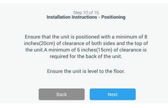
Figure 21. Installation Instructions (Positioning) Screen
