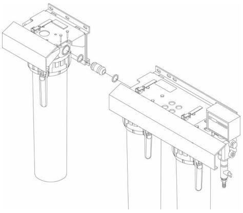
Figure 6-1. Three Holder System (3 Water Treatment Cartridges)
