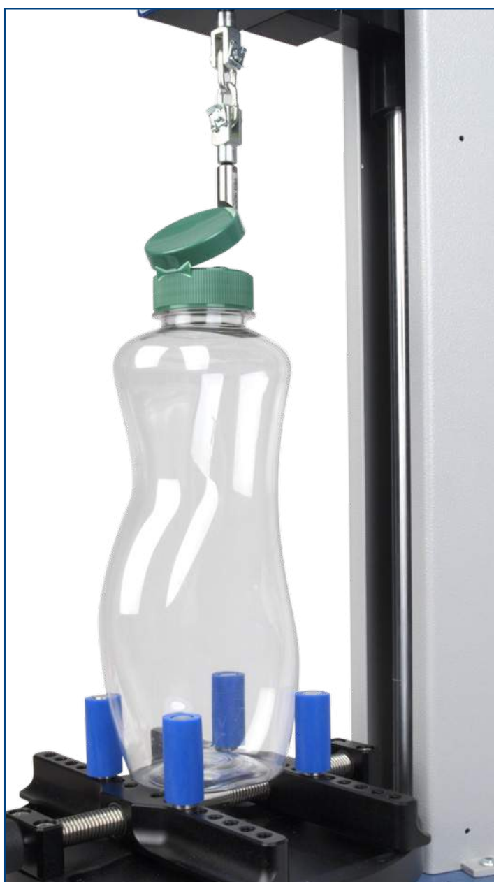
▲ 432-411 Large 4-peg container holder, plastic bottle application
