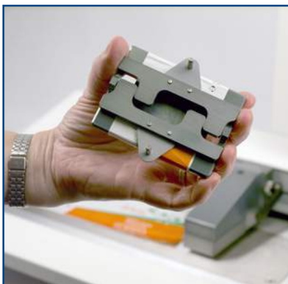
▲ 432-638: 200 g foam faced: ASTM D1894, ISO 8295
