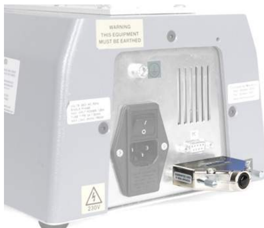
Rear panel with Digital I/O Loop-back Plug inserted
