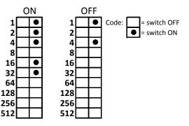
$\frac{32}{4+1} + \frac{1}{2} + \frac{1}{2} = 55 \text{ minute ON delay}$  $\frac{4+1}{4} = 5 \text{ minute OFF delay}$
