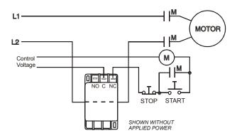
**FOR OVER-CURRENT ALARM CIRCUIT:** use the normally open contact. This will close on over-current, sounding the alarm.
