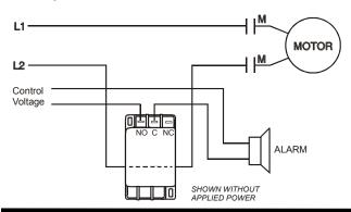
**FOR UNDER-CURRENT SENSING:** reverse the contact connections as stated above (use the normally open contact for load shutoff, or the normally closed contact for alarm).
