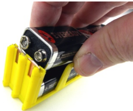
Figure 6 – slide battery in observing polarity
