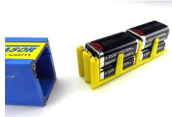
Figure 8 – slide battery sled back into case, closed end first
