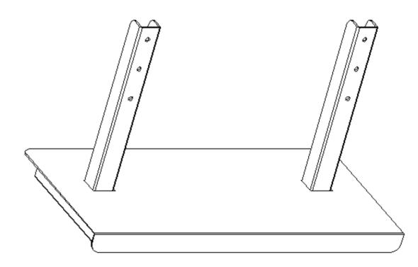
2. Assemble the stand and supporting upgright. Align the sliding groove, and slide in the stand then tighten the securing bolts.
