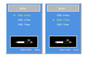
Press "enter" and "▲" or "▼" to select, and to move the OSD position in horizontal, or, vertical direction.
