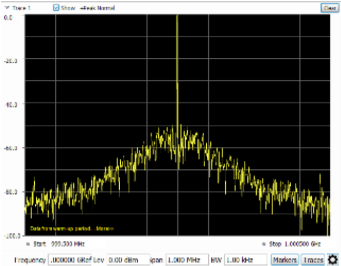
CW Signal output at 1GHz and 0dBm level
