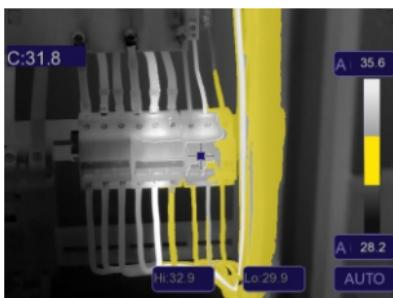
⌚ **Visible Zone:** The temperature between the high alarm and the low alarm set value will be colored to the palette, other part of the image will displayed as visible image.
