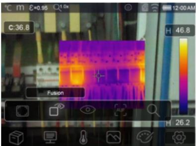
⌚ **AUF:** Auto Fusion mode, compare the centre area temperature with full screen, the machine will calculate the mix ratio of infrared and visible images automatically.
