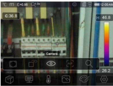
⌚ **Fusion:** Display fusion image of infrared and visible images.
