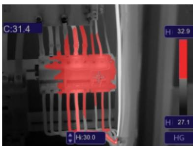
⌚\* **Low Alarm:** The temperature lower than the low alarm set value will be colored to blue, Press the Lo: 29.4 value button to adjust the below temperature.
