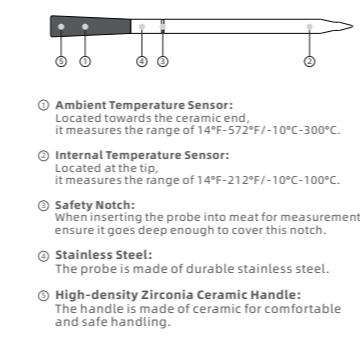
**Ambient Temperature Sensor:** Located towards the ceramic end, it measures the range of 14°F-32°F/-10°C-30°C.
