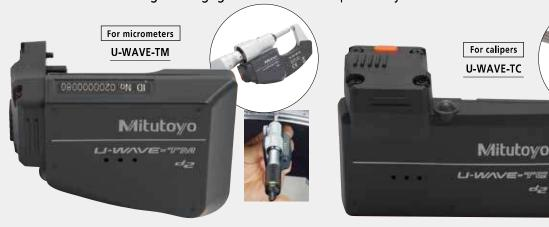
U-WAVE-TM for micrometers and U-WAVE-TC for calipers are available, both as the buzzer type and water/dust-proof IP67 type. The buzzer type notifies the normal reception of data by LED and buzzer sound. The water/dust-proof IP67 type is designed for a harsh environment and as such is only equipped with LED notification of data reception.
