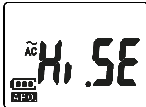
Figure 3-1 Vsense (high sensitivity) display
