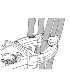
The unique wire separator allows you to easily separate and measure a desired wire in a bundle.
