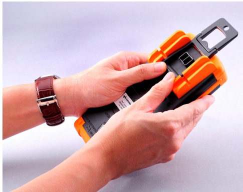
4. Re-attach the tilt-stand to an upright position
