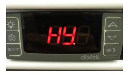
Press [UP] or [DOWN] until [CF] is displayed, press [SET] Change [C] to [F], and press [SET]. This changes Celsius to Fahrenheit
