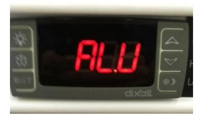
Then press [UP] or [DOWN] until [ALL] is displayed, press [SET] (Lower alarm setting) Change the value to [32] for factory setting, and press [SET]
