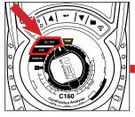
Rotate rotary dial to 02/Eff or AUX setting.
