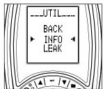
SETTING BACKLIGHT DURATION Rotate Roray Dial to MENU setting. Scroll to UTILITY selection Press ENTER ← button. Select duration: 15s, 30s, 45s, 60s, 300s Press ENTER ← button.
