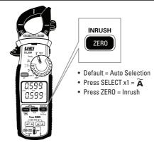
The UEi LRA Inrush is programmed to properly capture the starting current for compressor motors.
