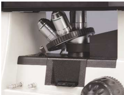
Close-up of the inverted nosepiece and objectives.
