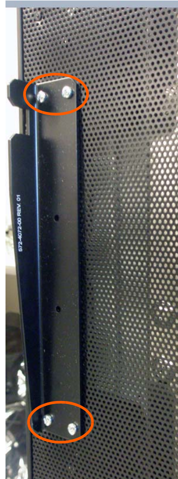
Portrait kickstand installed on display
