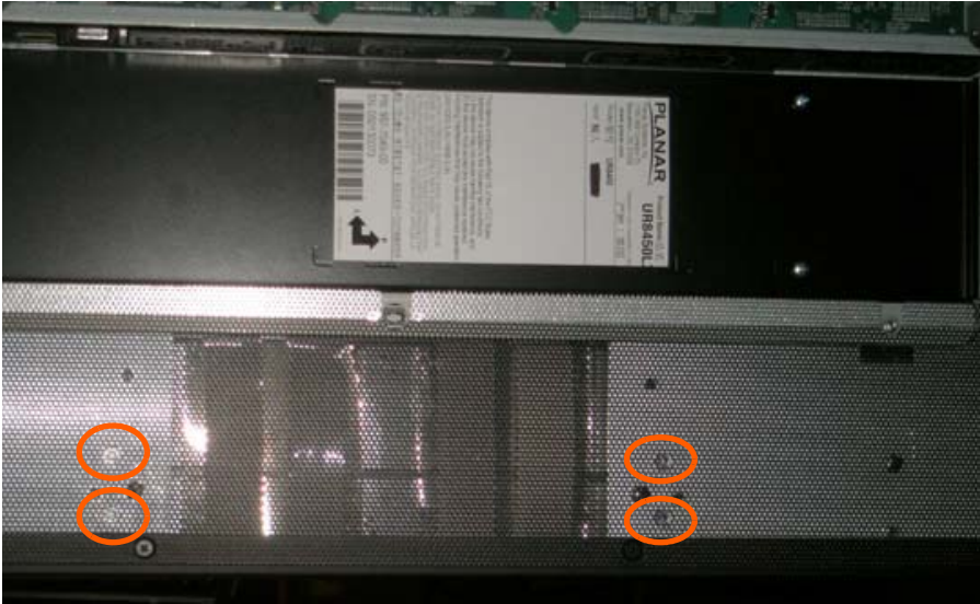
Landscape holes for kickstand bracket installation
