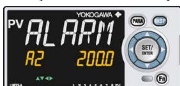
6. Press the SET/ENTER key to register the setpoint (the setpoint stops blinking).
