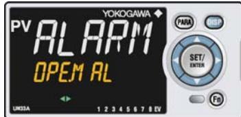
2. Press the SET/ENTER key to display the [A1] Parameter Setting Display.
