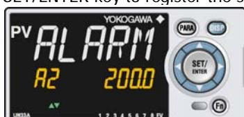
7. Press the SET/ENTER key to register the setpoint (the setpoint stops blinking).
