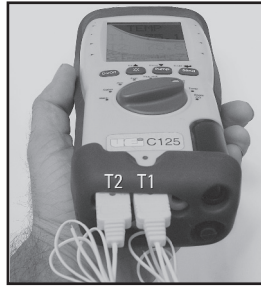
Connect flue probe thermocouple or accessory thermocouple connector to T1. Connect accessory thermocouple probe to T2. Compatible with any K-Type thermocouple probe or clamp.
