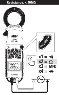
A Do not measure resistance on a live circuit.
