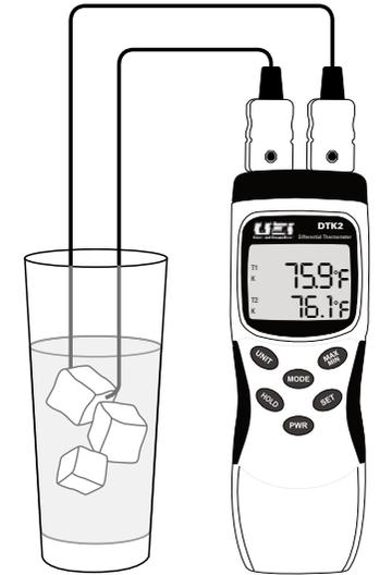
The DTK2 has an automatic ice-point calibration function. Please follow these steps to calibrate your meter to the thermocouple probes.
