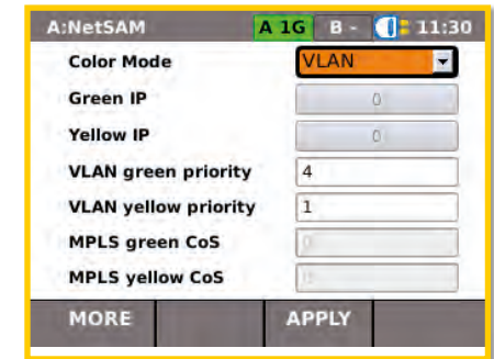
Checking VLAN priority set in Y.1564 (NetSAM) colour
