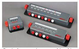
UNICO offers the 3 most popular counters: 2 key, 5 key with total window, and 8 key with total window. The 5 and 8 key models are sold with a WBC maturation series picto-strip just above the key windows. All metal housing is durable, chemical resistant, and easy to clean and disinfect. Signal bell when 100 cells have been counted.
