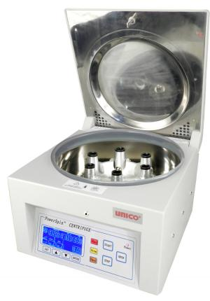
The all digital front panel with 3 pre-programmed options makes it easy to select most commonly run settings. The oversized display shows status, time, speed (RPM) and RCF (g). Precise speed control enables you to comply with CLIA recommendations for specific specimens.
