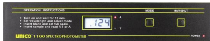
Close-up view of S1100 instrument panel
