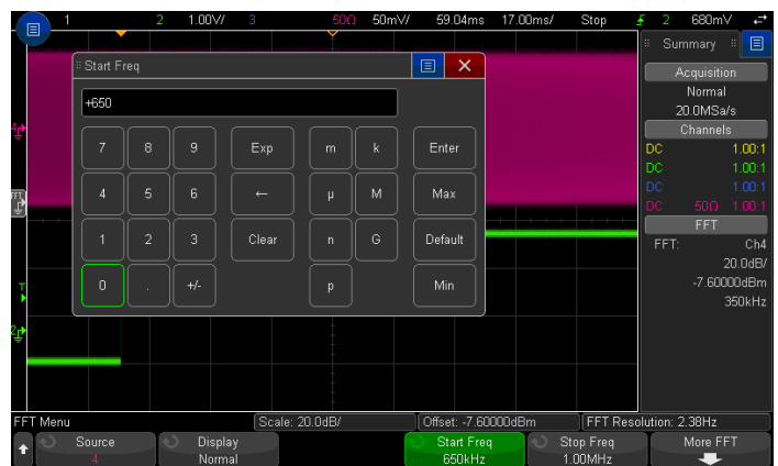
Figure 2. Use the keypad on the capacitive touch screen to enter values for start and stop frequencies.
