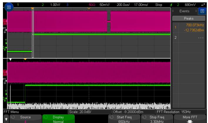
Figure 3. Time gated FFT, calculating the FFT only in the time specified window.
