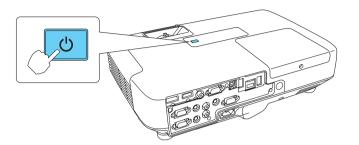
**Note:** To shut down the projector, press the  $\bigcirc$  power button twice, then unplug it. You don't have to wait for the projector to cool down.
