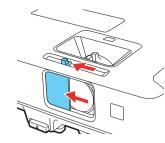
4 Press the  $\bigcirc$  power button on the projector or remote control. The projector beeps, the Status light flashes blue, and then stays on.
