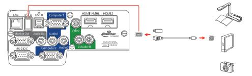
If you connect a digital camera, USB flash drive, or USB storage device, you can use the projector's PC Free feature to project images. You can also connect other Epson document cameras to the projector. See the online *User's Guide* for details.
