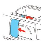
4 Press the  $\bigcirc$  power button on the projector or remote control. The projector beeps, and the Status light flashes blue and then stays on.
