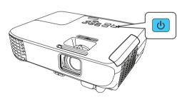
**Note:** To shut down the projector, press the power button twice.
