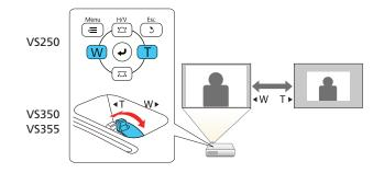
4 To sharpen the image, turn the focus ring.
