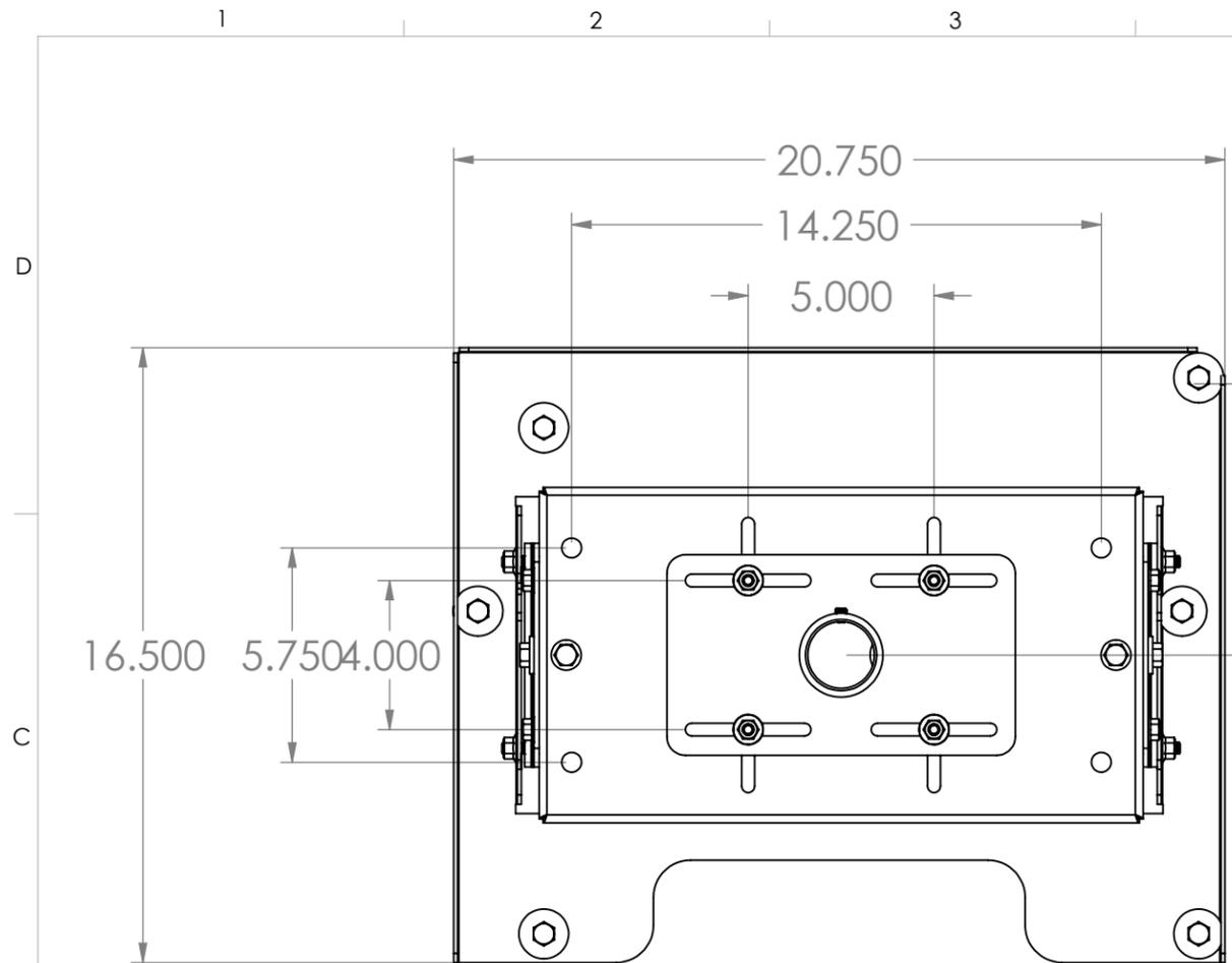
TOP OF MOUNT HAS 3" OF LATERAL SHIFT AND 3" OF FORWARD AND BACK MOVMENT BUILT IN.
