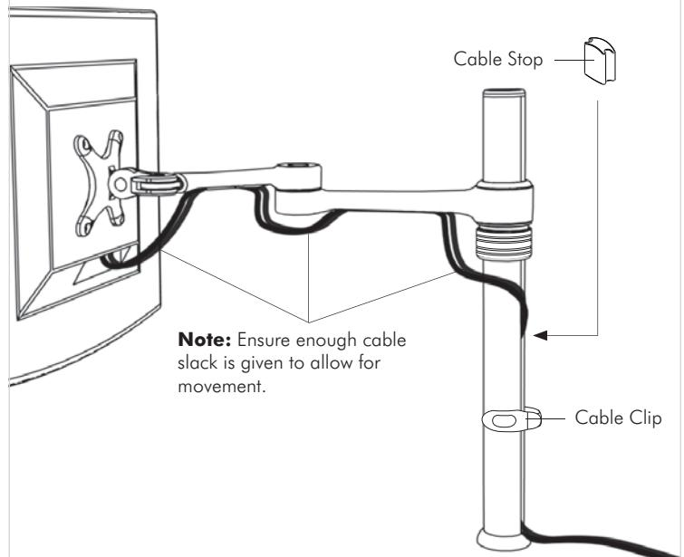
**Note:** Ensure enough cable slack is given to allow for movement.
