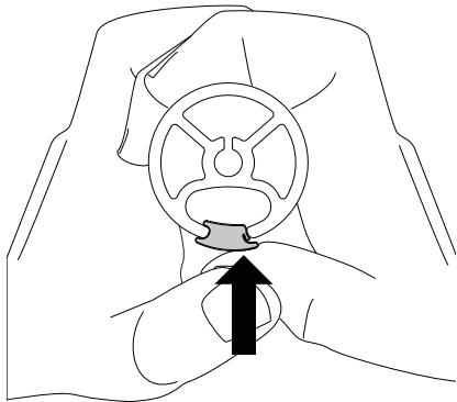
**B.** Press down firmly onto the other edge of the Cable Stop and hold. This allows the rear profile to flex in place.
