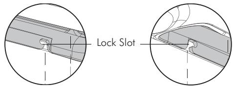
**A.** Insert Cable Covers up into Lock Slots.
