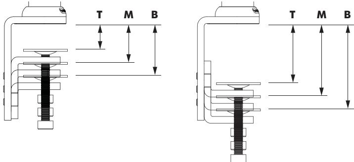
**2.4** Remove the M8 x 16mm Socket Head Countersunk Screws to release the Desk Clamp Bracket.
