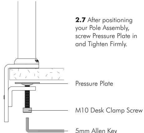
**2.7** After positioning your Pole Assembly, screw Pressure Plate in and Tighten Firmly.
