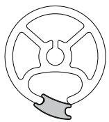
**A.** Insert Cable Stop on one edge of the Pole Slot.
