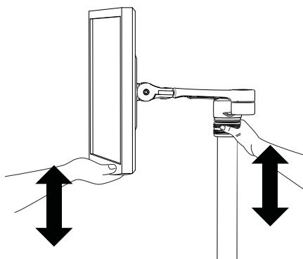
**5.2** Lift/Lower the Screen to the desired height. Move both Screen and Arm assembly together.
