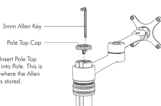
**3.4** Insert Pole Top Cap into Pole. This is also where the Allen Key is stored.
