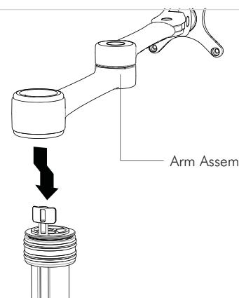
**3.2** Slip the Arm Assembly over the Handgrip Tab and then onto the Pole.
