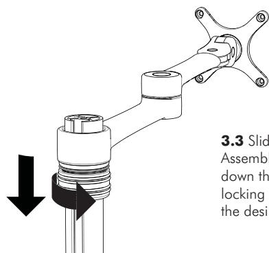
**3.3** Slide the Arm Assembly and Handgrip down the pole before locking the handgrip at the desired height.
