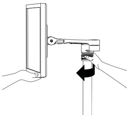
**5.1** Unlock Handgrip ensuring both the screen and arm assembly are supported.
