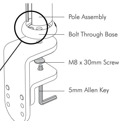
**Note:** Ensure that the Slot Tab in the Bolt Through Base fits snugly into the Slot on the Pole Assembly.
