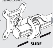
If necessary, adjust the tension between the Donut and the Pole using the 5mm Allen Key supplied.
