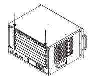
4. Tighten the two screws on the VM7104 board to fasten it to the Modular Matrix Switch, until it's secured to the unit
