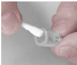
Figure 4. Cleaning Lamp Window
